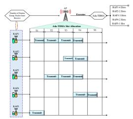
Figure 2: Ada-TDMA based Time Slot Allocation
